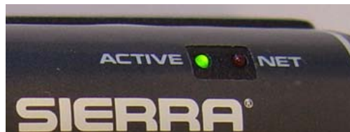
LED's showing the activities of the Compod™
